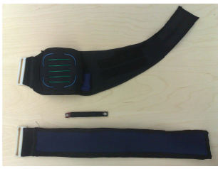
(a) Thigh enclosure (top), Bend sensor (middle), Calf enclosure (bottom)
