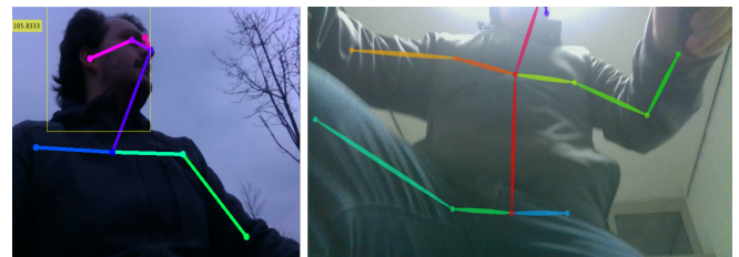
Figure 3. Recognition of head movement (left) and hand gestures (right) of cyclists using the OpenPose library.
