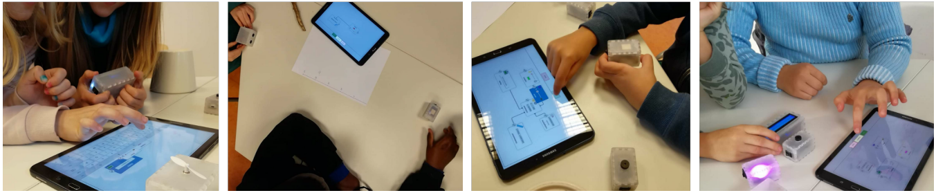
Figure 5: Different examples of toolkit use (from left to right): using the motor module with the distance sensor to make a nail polish dryer, understanding the distance sensor using a reference paper-based ruler, combining multiple modules for an alarm system, and creating a game by combining three feedback modules (LCD-text, sound-module and multi-color light).
