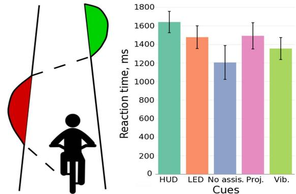
**Figure 7: Accumulated trajectory error left and right: red area indicates trajectory error to the left and green – to the right. We summed these areas along the cycling trajectory, estimating an accumulated trajectory error for each side (left). Reaction times to the visual search task for the lane keeping cues (right).**
