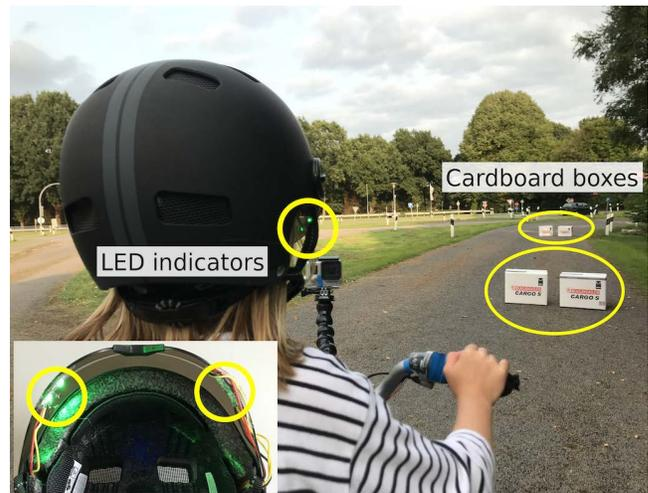
Figure 1: The LED helmet and road obstacles used in the controlled test-track experiment.
