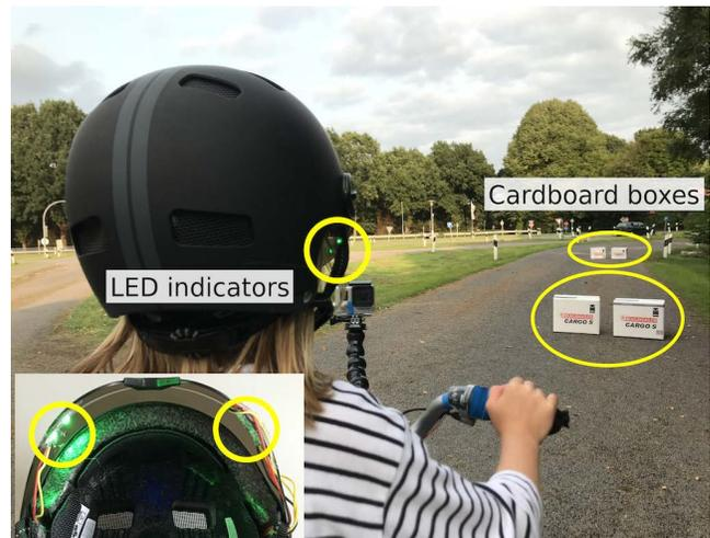
Figure 1: The LED helmet and road obstacles used in the controlled test-track experiment.
