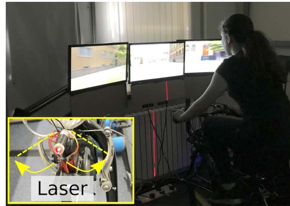
**Figure 5: Laser projection: we mounted a laser on a servo in front of the bicycle to indicate lane keeping cues by turning it left or right and projected a line under the screens.**
