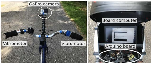
**Figure 8: A tricycle equipped with a laptop in the rear cargo box, vibrotactile feedback on the handlebar, and a GoPro camera for in-field observations.**
