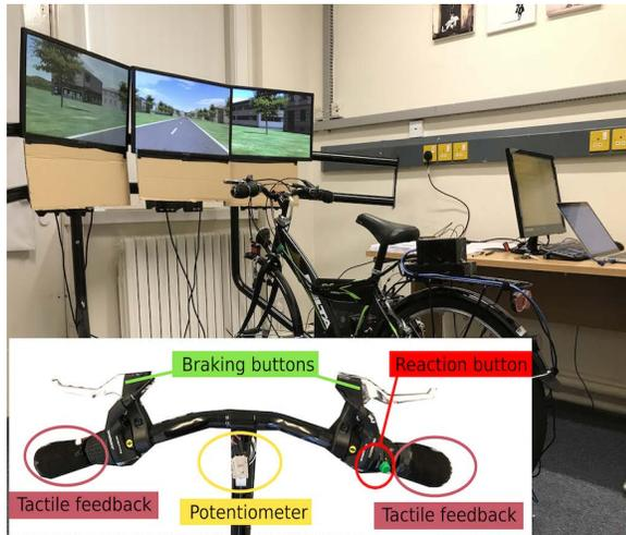
**Figure 4: Bicycle simulator: handlebar with tactile feedback and a bicycle mounted on the platform with Hall effect sensor, magnets for measuring speed, servo with laser in the front and microcontrollers.**
