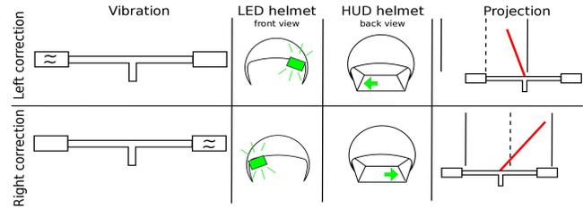
**Figure 3: Overview of encodings for the lane keeping cues used for trajectory corrections. Children experienced each cue via vibration on the handlebar, blinking light in the LED helmet, blinking arrows in the HUD helmet, and a projected laser line indicating left and right in front of the cyclist.**
