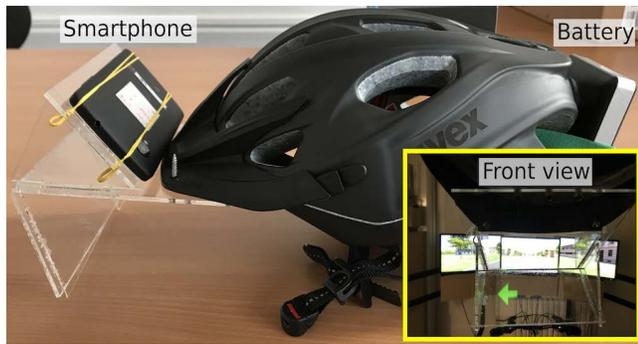
**Figure 6: HUD helmet: visual cues displayed on the smartphone were reflected in the plexiglas surface of a holder in the front. A battery power bank at the back was used to balance the weight and charge the smartphone.**
