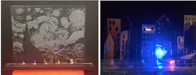
Figure 7. Laser engraved pattern of “Starry Starry Night” with five LEDs installed into standing slot (left), and two overlaid laser cut frames of skyline with blue/yellow enabled (right)
