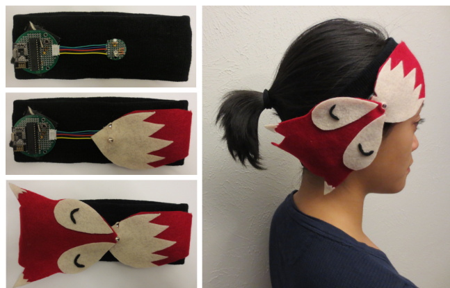
Figure 7. UV wearable device crafted into a fox themed headband with felt, velcro and fabric glue.
