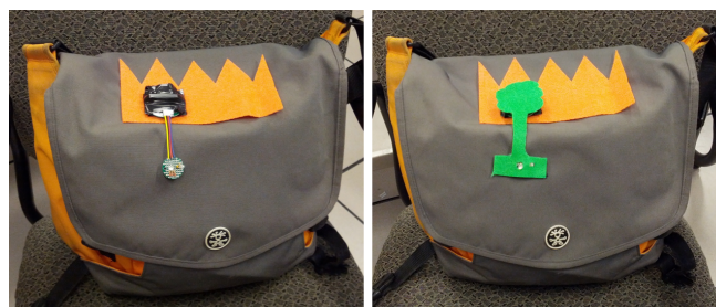
Figure 6. UV wearable device crafted into a messenger bag with felt, velcro and electric tape.
