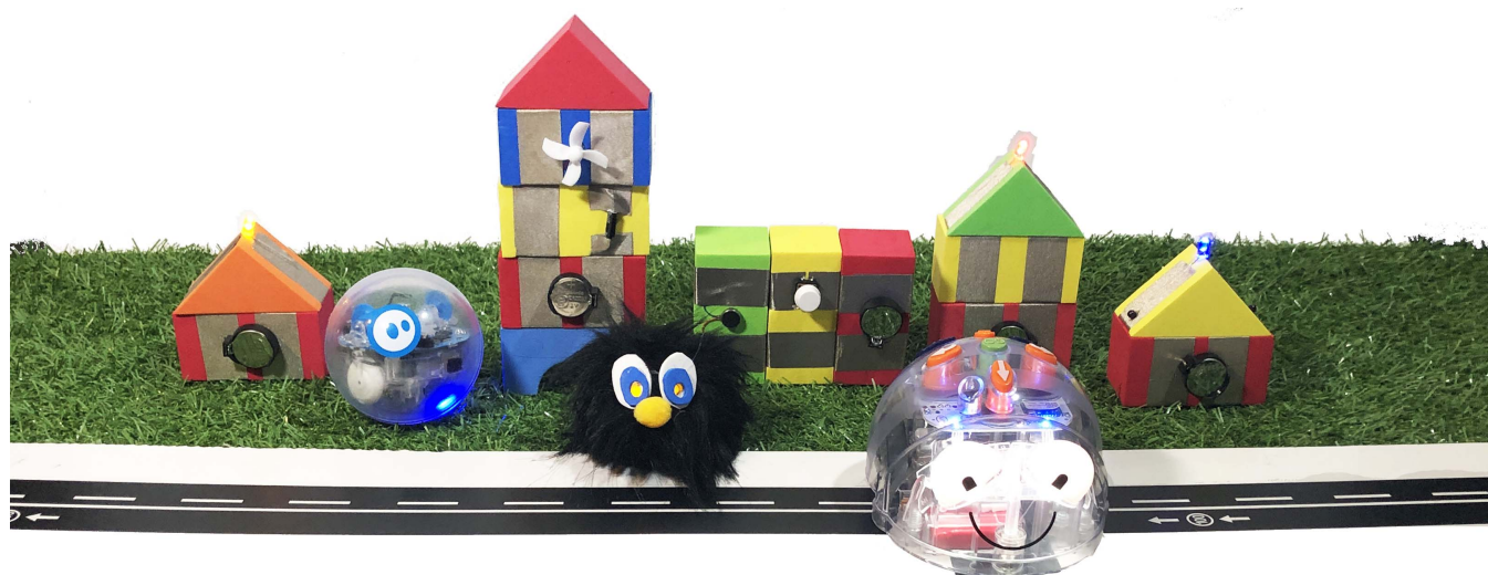
Figure 1: An electronics and programming package for people with intellectual disabilities consisting of TapeBlocks, Blue-Bot, and Sphero. These technologies were used in combination with common craft materials to explore making of unique artifacts and creative experiences.
