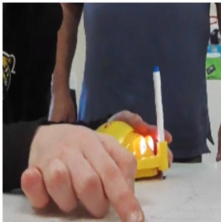
(a) A Bee Bot being programmed to draw a smiling face with a pen attachment.
